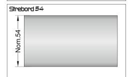
Strebord 54<sup>®</sup> Is a homogenous solid sheet of 54mm thick graduated density particleboard (minimum density 530kg/m³ to maximum density 630kg/m³).
