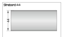
Strebord 44<sup>®</sup> is a homogenous solid sheet of 44mm thick graduated density particleboard (*minimum density 530kg/m³* to *maximum density 630kg/m³*).
