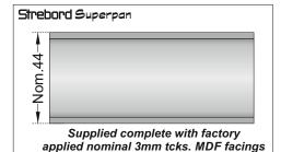
Strebord Superpan® Is supplied as a homogenous solid sheet of 38mm thick graduated density particleboard (minimum density 560kg/m³) complete with factory applied nominal 3mm thick MDF facings. The facing is bled into the core rather than flat bonded, variances can be experienced due to the manufacturing process. Where required, (by reference to relevant sections in this manual), door leaves must be lipped in hardwood.
