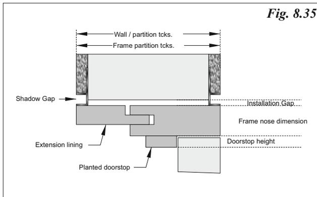
**Frame Designs without Architrave:** For frame designs using a 'shadow gap' the doorset should be installed before the application of the final wall / partitioning finishing with a dry lining option being recommended to minimise the risk of moisture or plaster contamination of the door frame.
