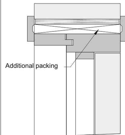
For some performance doorsets e.g. fire rated and sound attenuating doorsets, additional packing is required at the head of the doorset where the doorset height is reduced to suit floor conditions.
