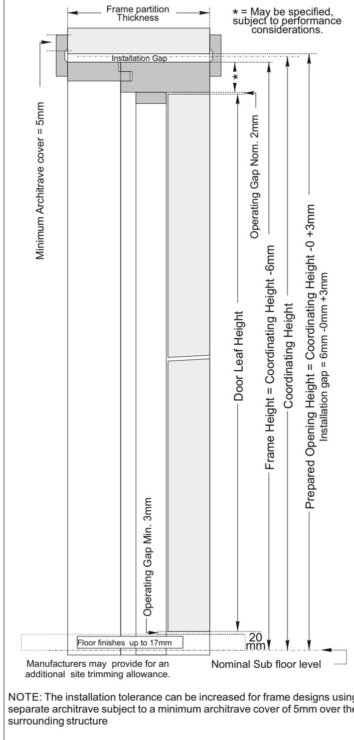
NOTE: The installation tolerance can be increased for frame designs using separate architrave subject to a minimum architrave cover of 5mm over the surrounding structure
