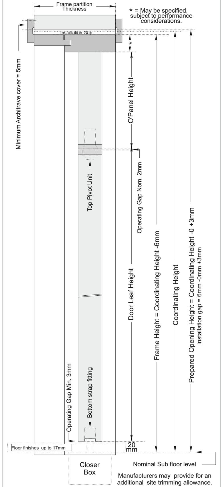
Storey Height Doorsets - Double Action - with Flush Over panel - Single leaf doorsets.
