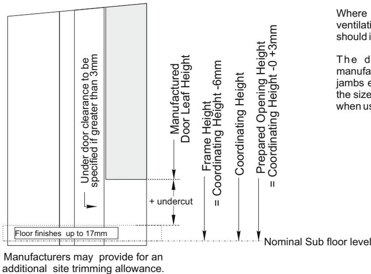
Where a large undercut is required e.g. for ventilation, the specifications / project details should identify this requirement.
