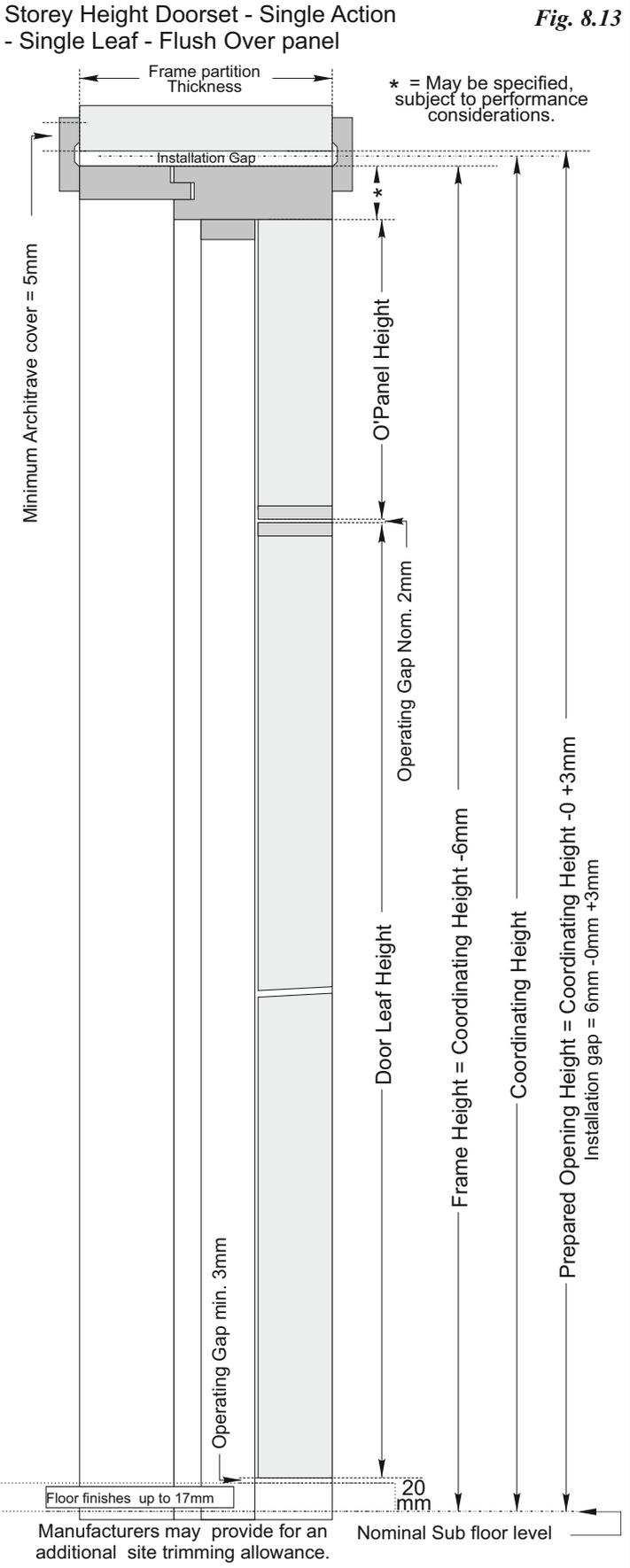
Storey Height Doorsets - Single Action - with Flush Over panel - Single leaf doorsets.
