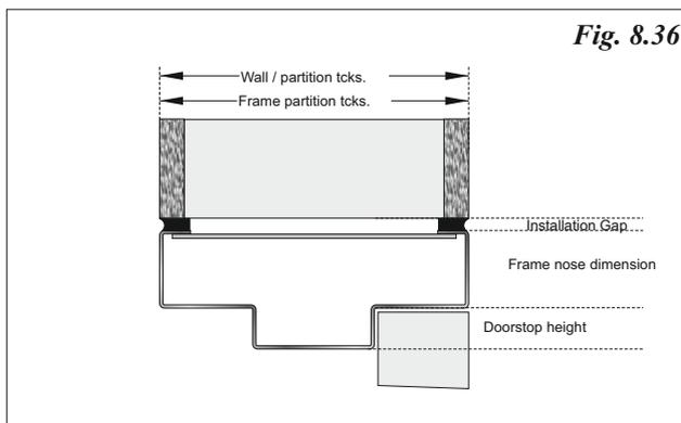
**Metal Frames:** Most metal frame, particularly steel frame designs do not include architrave. Considerations related to frame with 'shadow gaps' will generally apply.
