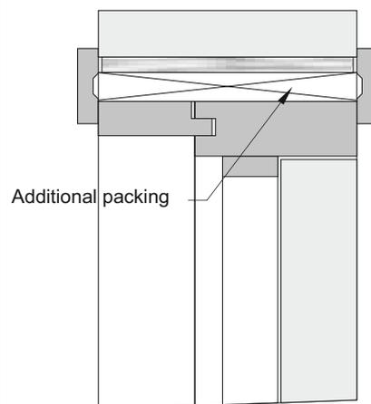
For some performance doorsets e.g. fire rated and sound attenuating doorsets, additional packing is required at the head of the doorset where the doorset height is reduced to suit floor conditions.
