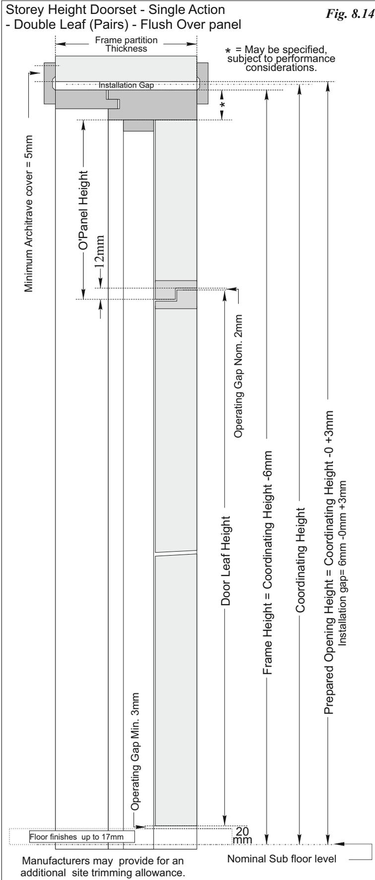
Storey Height Doorsets - Single Action - with Flush Over panels - Double Door Doorsets (Pairs).
