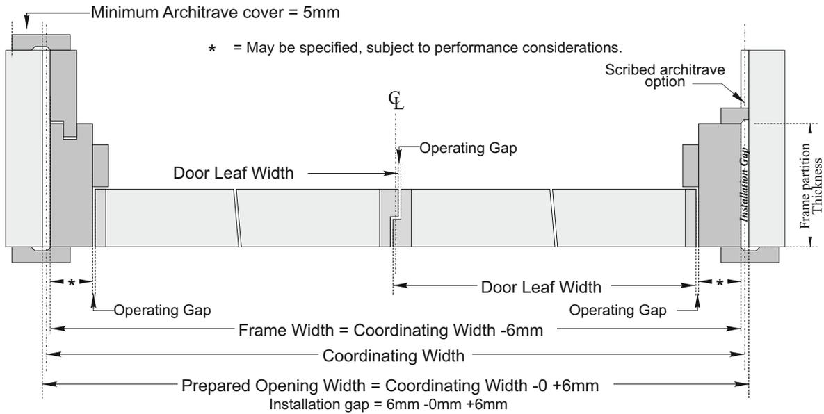
NOTE 1: The installation gap can be increased for frame designs using separate architrave subject to a minimum architrave cover of 5mm over the surrounding structure.
