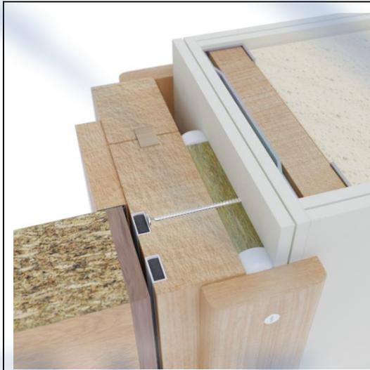
Split frames are permitted providing that both frame sections are secured to the wall in accordance with section 11.5. Furthermore, the main frame section (from which the door is hung) must be constructed to at least the minimum door frame section size (width and depth) as per the requirements noted in this report – see door frame section. The extension piece must be constructed using the same timber species as the main frame section.
