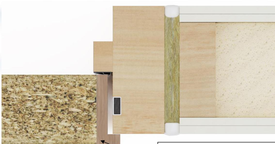
**Fig. 5 – Over rebated edge detail**
