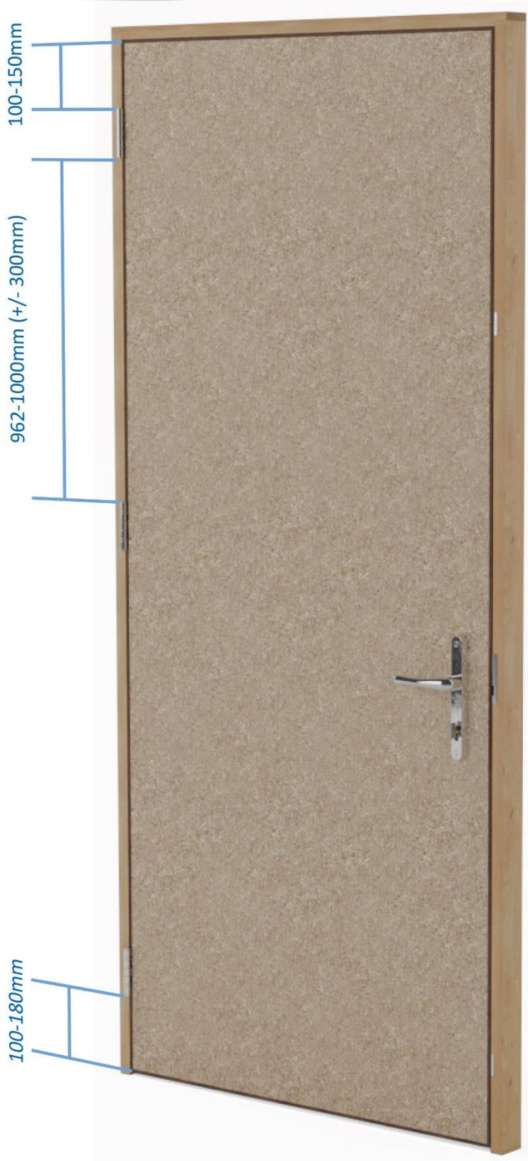
**Fig. 14 – Drawing showing approved hinge positions**
