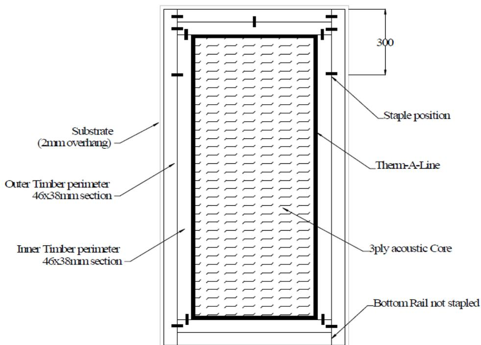
5. Coat one substrate with Apollo A7561 adhesive (140Kg/m<sup>2</sup>) and over mist with water (5% of the adhesive weight used). Avoid excessive water. Alternatively PVA-D3 may be used in lieu of the Apollo adhesive. Place (adhesive side up) on pressing platform
