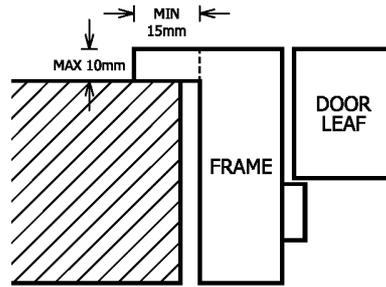
**Figure 1. Frame option with integral architrave**
