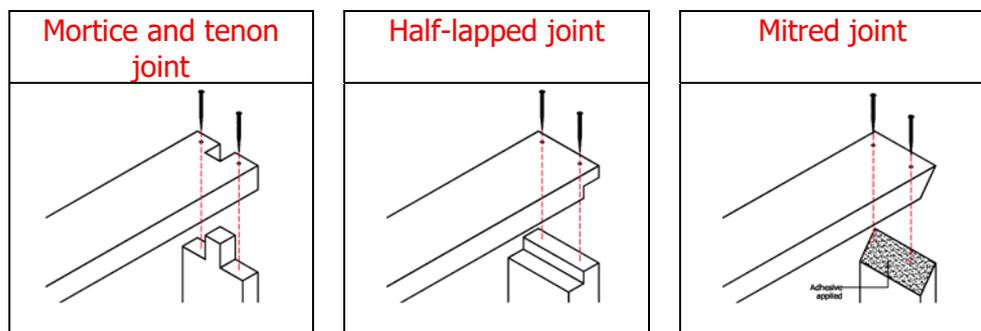
**Figure 2. Head/Jamb jointing options**
