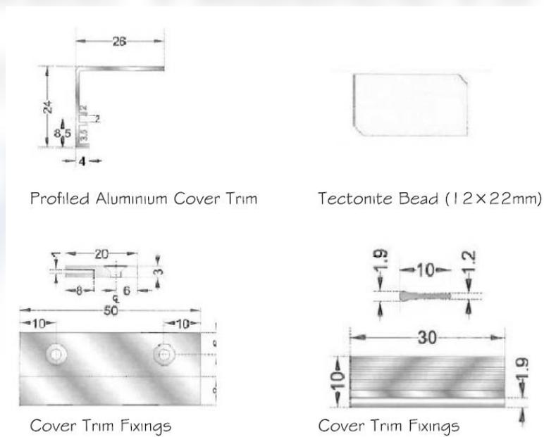
Figure 6 - Glazing system option 2 components
