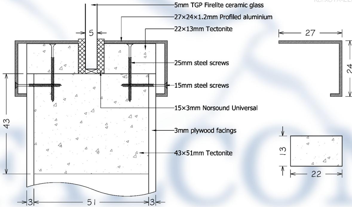
Figure 9 - Glazing system option 5 assembly and components
