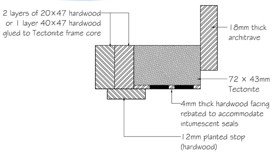
Figure 3 - Tectonite (hardwood composite) door frame
