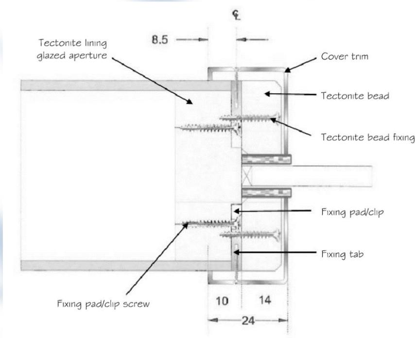
Figure 5 - Glazing system option 2 assembly
