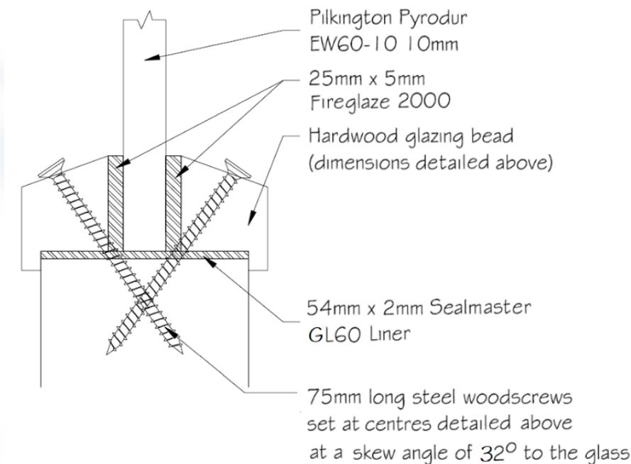
Figure 8 - Glazing system Option 4 bead detail
