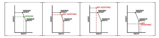
Field of Application for 44mm Thick Moralt LAMINESSE FireSound FD30 Timber Door Leaves Installed in Timber Frames in Accordance with BS476: Part 22: 1987
