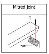
Architraves : Where the face of the frame, and the door, are flush with the face of the wall, loose architraves are optional, and have no fire performance requirements, and so can be freely specified, subject to adequate fire stopping. (See Section 3.8 regarding wall/frame gaps).
