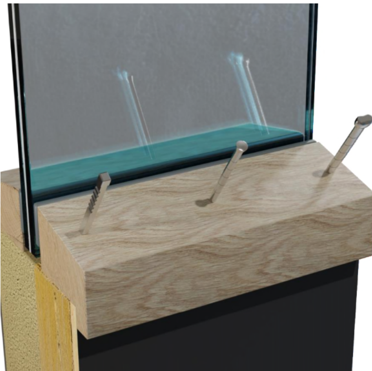
Fig 7 – 3-D cross section depicting round, oval and rectangular pins
