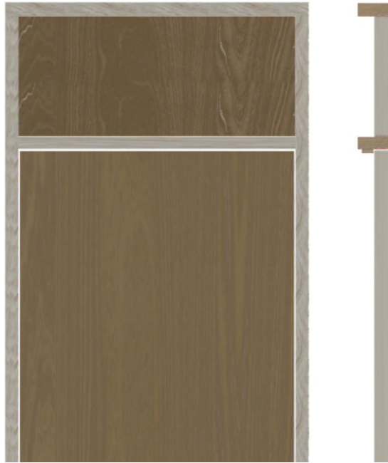
Fig 3 – Front elevation and cross section of a single leaf door with over panel
