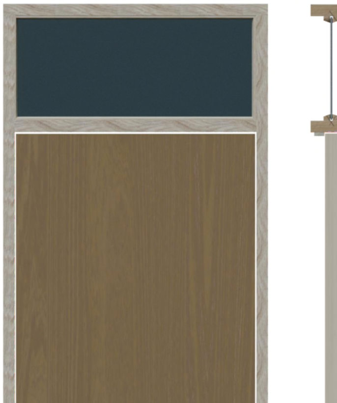
Fig 5 – Front elevation and cross section of a single leaf doorset with fanlight
